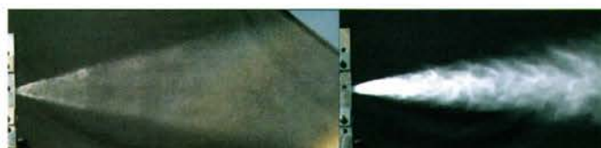
Figure 2: Left: Standard pressure atomiser captured @10,000 fps. Right: High energy micro mist captured @10,000 fps.
