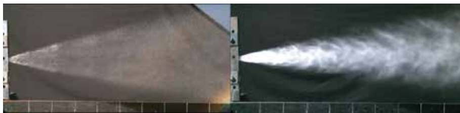
Nozzles ain't nozzles: (left) standard pressure atomiser captured @10,000 fps; and (right) high energy micro mist at 10,000 fps.
