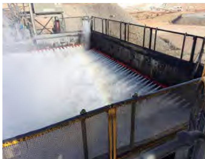
Micro-mist dust suppression system around ROM crusher bin at Karara mine.
