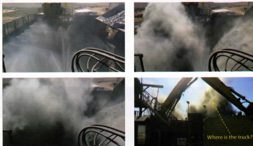
Figure 2: Excessive Dust Emissions with Existing Water Spray System (1000 L/min).
