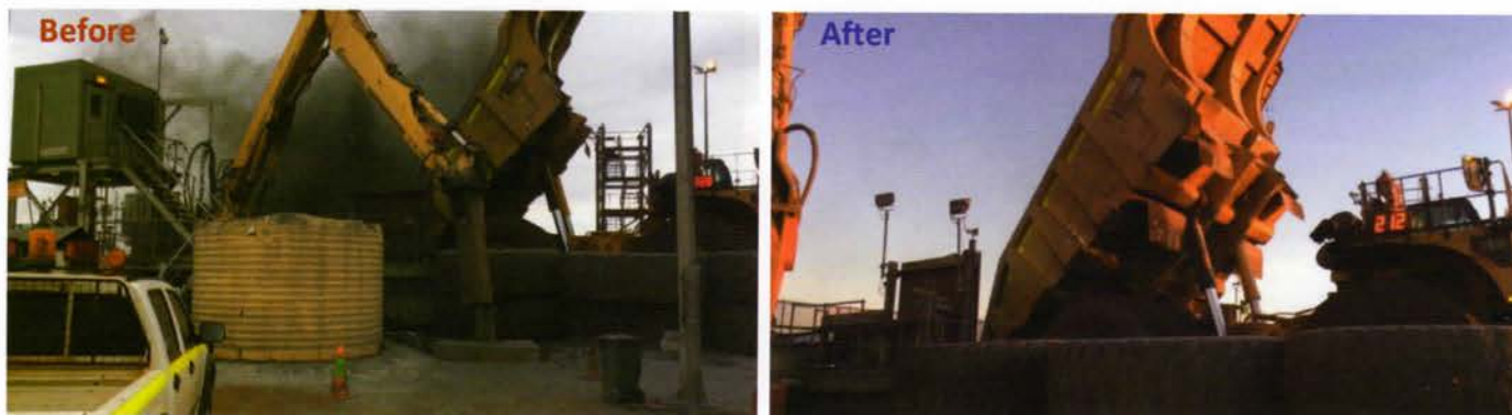
Figure 7: Comparison of old Water Spray System (left) and new Enviromist Dust Suppression System (right).
